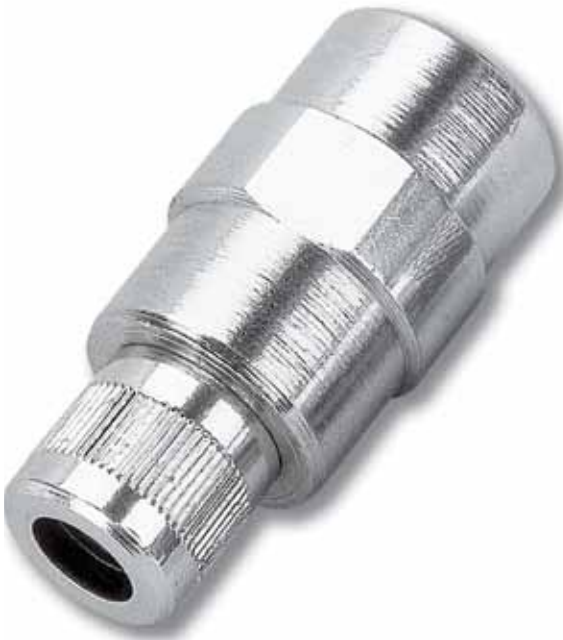
443-61 Universal Bulk Loader Valve This dual-purpose adaptor can be used with both 9 mm Straight & American Tapered 0.58" (14.7 mm) Bulk Loader Valves The top sleeve adapts to 9mm straight loader valves, which may be removed, and the base used with the larger 0.58" (14.7 mm) loader fittings
